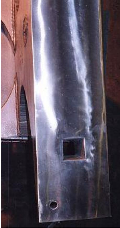
I should have made the Pritchel hole the same way as the Hardie. It is very hard to drill through the hard face - almost impossible.
