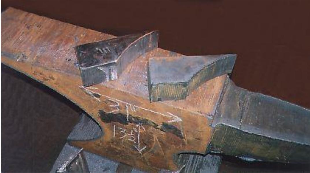
After you have the cut blank profile, you have to do a couple of bevel torch cuts by hand to give the shape to the horn.
