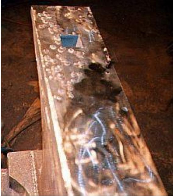
It usually takes 2 or 3 cycles of welding and grinding to get all the bubbles out.
