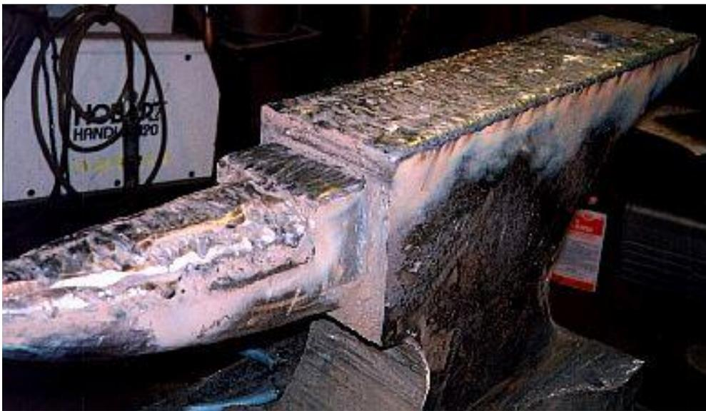
When hard facing the sides, I go about 1-1/2" down and run a simple bead to act as a guide. [Side Facing](#)
