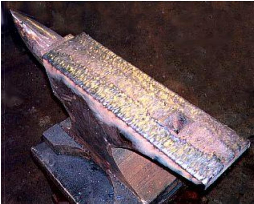
Hard facing completed on the anvil horn and shelf. [Horn and Shelf](#)
