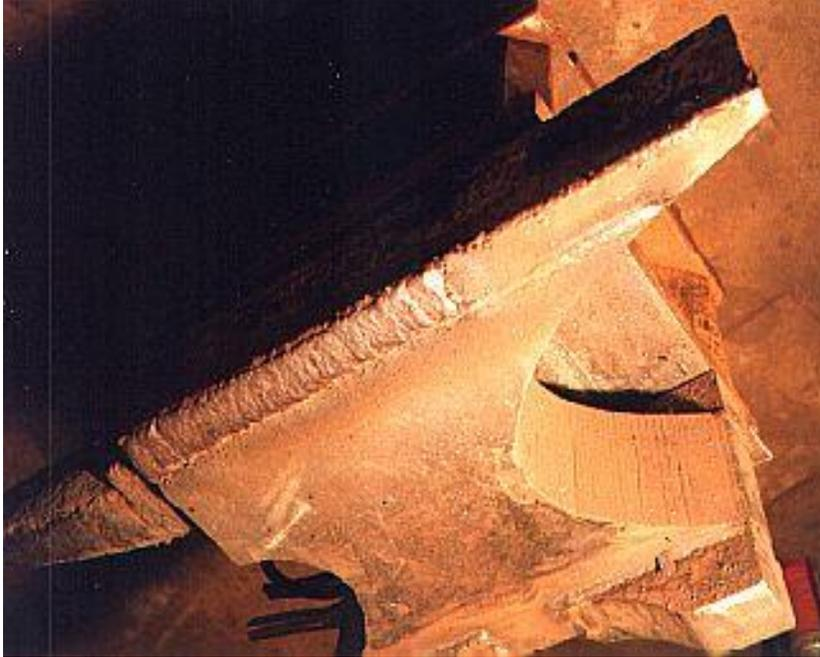
This view shows the completed hard facing of the side and horn side. [Side View](#)
