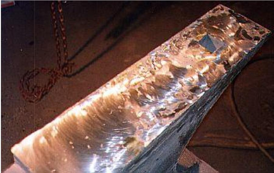
If you use a cup wheel on a 7 inch or 9 inch Right Angle grinder you will find it easier to get a flat face. You will want a wheel designed for hardened or alloy steels that cuts fast. For the final polishing of the surfaces invest in some "flapper" style sanding wheels of say 40, and 80 grit. On a 4-1/2 inch right angle grinder they are just great for finishing.
