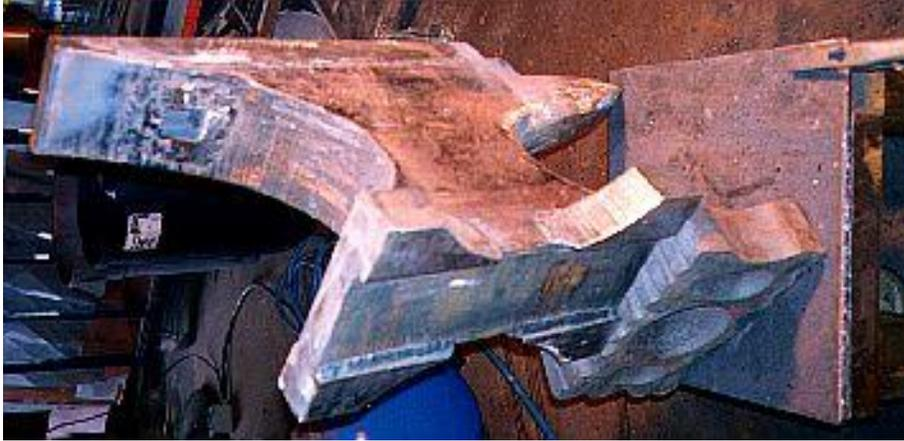
View showing the finished second pass of the hard facing with more edge buildup. Notice how the hardie hole sticks up through all the hardsurfacing. [Top Hard Surface View](#)
