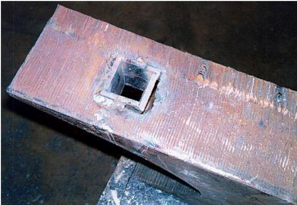
You can drill 1 or 2 pritchel holes, depending on your preferences. I like to have either one hole 3/8" Dia.. or 2 holes, 5/16" and 1/2" diameter. These are drilled so there is about 3/8" of steel left to the edges of the heel. Pritchel holes are used for punching holes, bending small bar stock, and mounting plates. If the holes get filled with hardfacing it is possible to clean out the hardfacing with a cutting torch from the underside.
