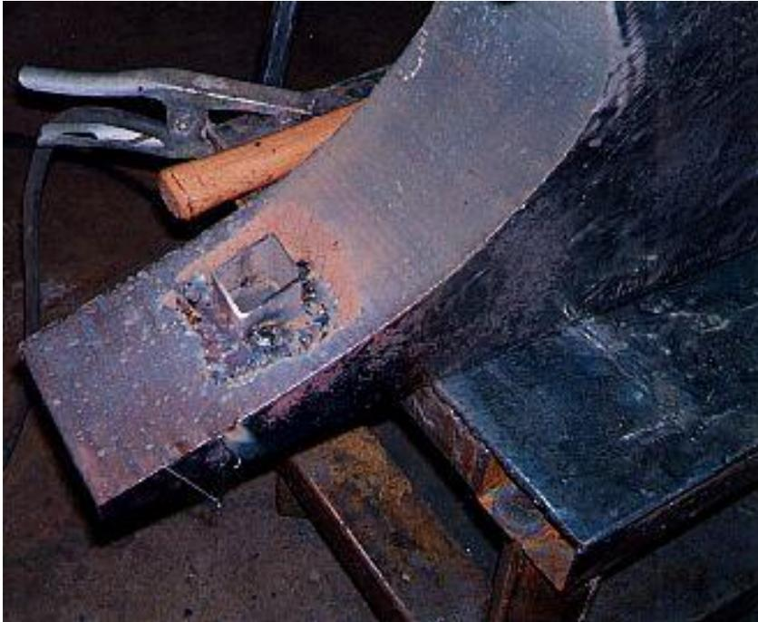
This view shows the short length of 1-1/2" X 1-1/2" thin wall steel tubing that was used to bring the bottom of the Hardie Hole flush with the bottom of the heel. [Bottom View w/Tubing](#)
